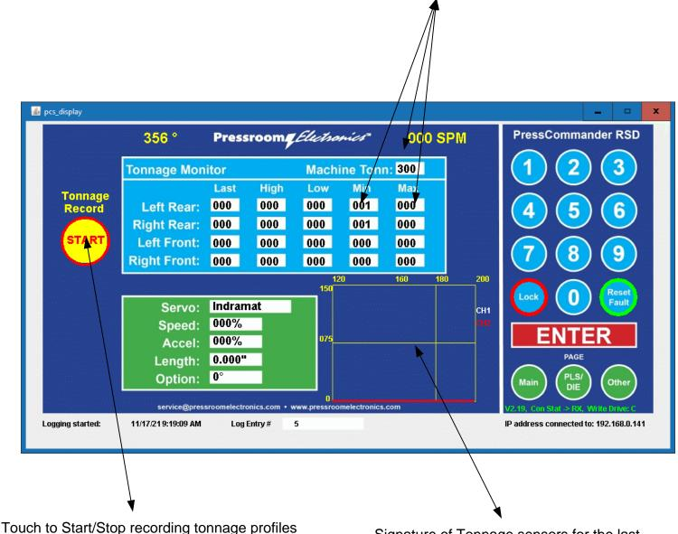
Touch to Start/Stop recording tonnage profiles to a CVS spreadsheet. 100 cycle max
